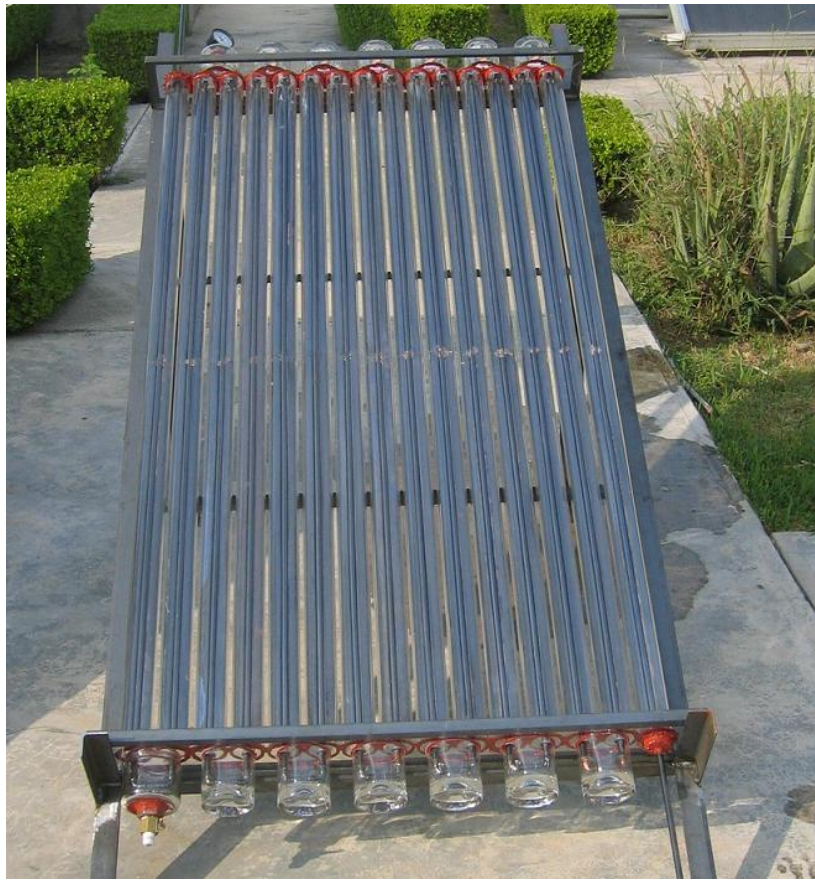
Fig 11: First Prototype of the VCSC with segmented headers
